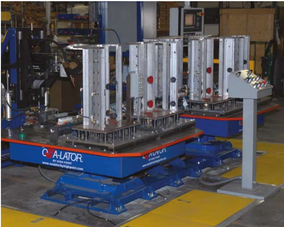
Contour-Arc CNC Spot Welding System, developed to produce various sizes and styles of end products with minimal changeover time. All functions are controlled by a Siemens SINUMERIK 802D solution line CNC. The system also features Siemens 1FK7 servomotors for high-accuracy positioning.
