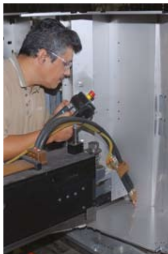
Contour-Arc CNC Spot Welding System, developed to produce various sizes and styles of end products with minimal changeover time. All functions are controlled by a Siemens SINUMERIK 802D solution line CNC. The system also features Siemens 1FK7 servomotors for high-accuracy positioning.
