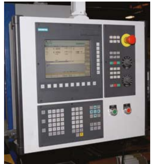
Contour-Arc CNC Spot Welding System, developed to produce various sizes and styles of end products with minimal changeover time. All functions are controlled by a Siemens SINUMERIK 802D solution line CNC. The system also features Siemens 1FK7 servomotors for high-accuracy positioning.
